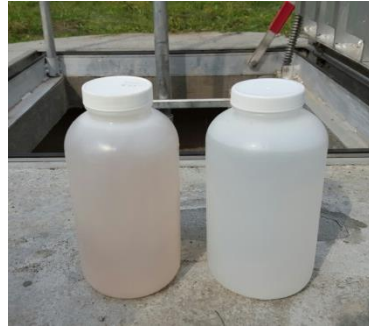
Figure 1 – Initial Testing Samples: Intake Pond Water on left, Treated Water returned to the pond on the right.
