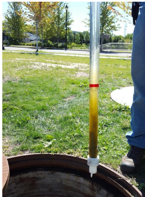
Figure 2 – Dissolved Phosphorus sludge collected from the bottom of the settling tanks.
